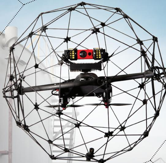
THE COLLISION-TOLERANT UAV
